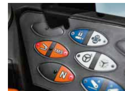
All functions are arranged simply and clearly on the backlit membrane keypad according to the tried and tested Fendt operating logic.
