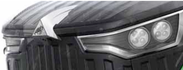
LED daytime running lamps and work lights integrated in the front of the bonnet including bonnet camera.
