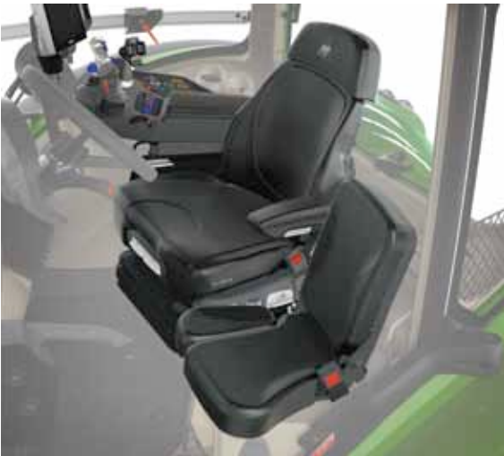
The new black leather version of the Dualmotion comfort seat with active suspension, the Fendt Evolution active, is especially classy and dirt-resistant – and always comes with a comfort passenger seat in leather.
